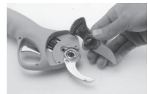
4. Unscrew the pin and remove the moving blade
