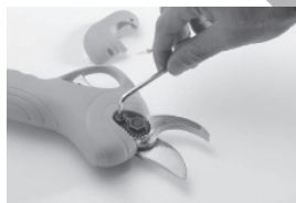
2. Remove the screws from the blade nut retaining buckle (this step is critical).
