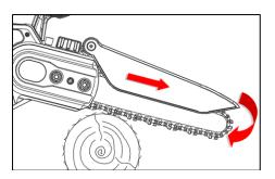
• When the guide plate is used for a bottom-up cut, the pushing direction of the saw is towards the operator.
