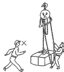
In case the hand chain pull force exceeds the normal, don't pull by increasing force. Stop operation immediately and inspect the hoist.
