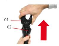
Before you put the head back on, we recommend lubricating the shaft with guide pin 01.
