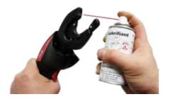
Spray the end of the head on the wire-pinching side.
