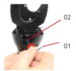
Once you have disconnected the tying head, remove the end-of-reel wire 01 from the tying head. You can also take the opportunity to insert the new wire, as it will be easier to thread through.
