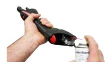
Spray directly on to the wire on the reel, once or twice per reel, to help the wire to slide more easily as it moves round the reel.
