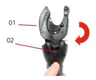
Take hold of tying head 01 and pull it to remove it from the body 02 of the machine.
