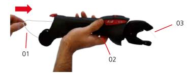
If the wire does not emerge, unclip lever 01 and pull it right out of the machine.
