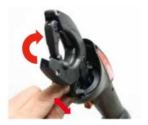
It is normal for the tying head 01 to resist and make you force it to bring it back into its operating position.
