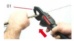
Go right up to the abutment to ensure that the arm closes fully and attaches the wire correctly.
