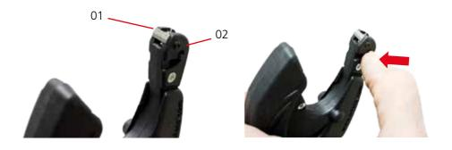
The wire may be bent at exit 01: **(no need to disconnect the machine)** simply go through the cycle empty or run the knife only and resume the tying action.
