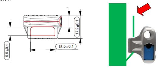
This will of course mean a variable fit with different metal posts. When using chains etc many end users will "tap" the tab on the metal post to close up the gap. This can also be done when using a VIT-S if necessary
