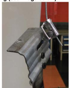
The metal tabs on the post were deformed to failure at just over 200kg. The Gripple is thus rated at a far higher load than the post is designed to encounter.
