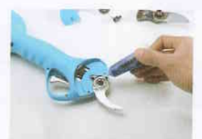
6. When replacing the blades, the blade pin shaft, swing gear, plane bearing and blade all need to add lubricating oil
