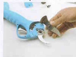
4. Disassemble the pin and remove the moving blade
