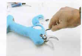
3. Disassemble blade nut
