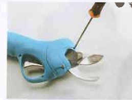
1. Disassemble the screws with a screwdriver and open the lid.
