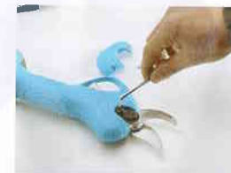
2. Disassemble the screws from the blade nut retaining buckle (this step is critical)
